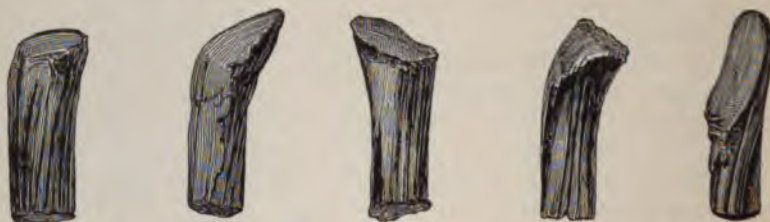
Fig. 106.—Deformation of small-caliber jacketed bullets (after Bruns).
